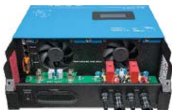
Inside the SmartSolar MPPT RS 450|100
